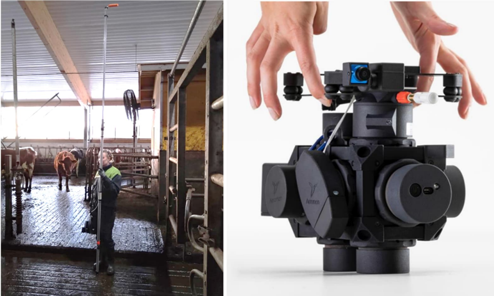
Figure 8. Lefthand side: Aeromon employee during indoor measurements holding a telescopic arm with a sample line and the measuring device. Righthand side: Picture of the Aeromon BH-12 measuring device. Figure reprinted with the permission of Aeromon Oy.
