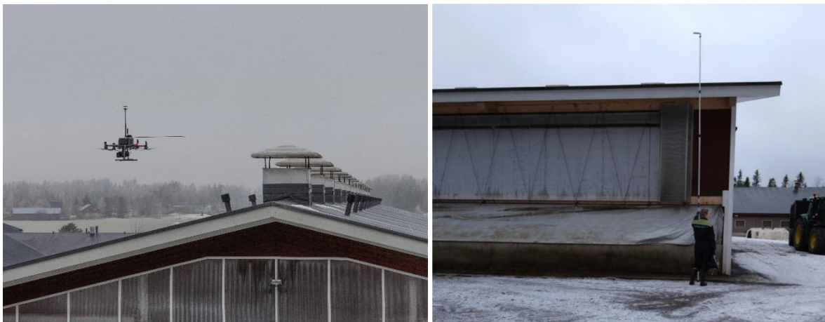
Figure 10. Lefthand side: Flight assisted measuring on the emissions using drone. Righthand side: Picture of Aeromon employee during outdoor measurements holding a telescopic arm and the measuring device.
