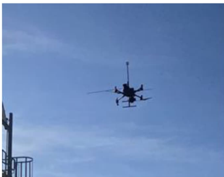
Figure 7. An anemometer on the roof of the drone.
