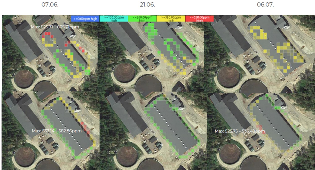
Figure 34. CO 2 levels inside and outside barn during summer season. Light green represents the background level which was measured to be 320 ppm). Top row: inside measurements. Bottom row: outside measurements.
