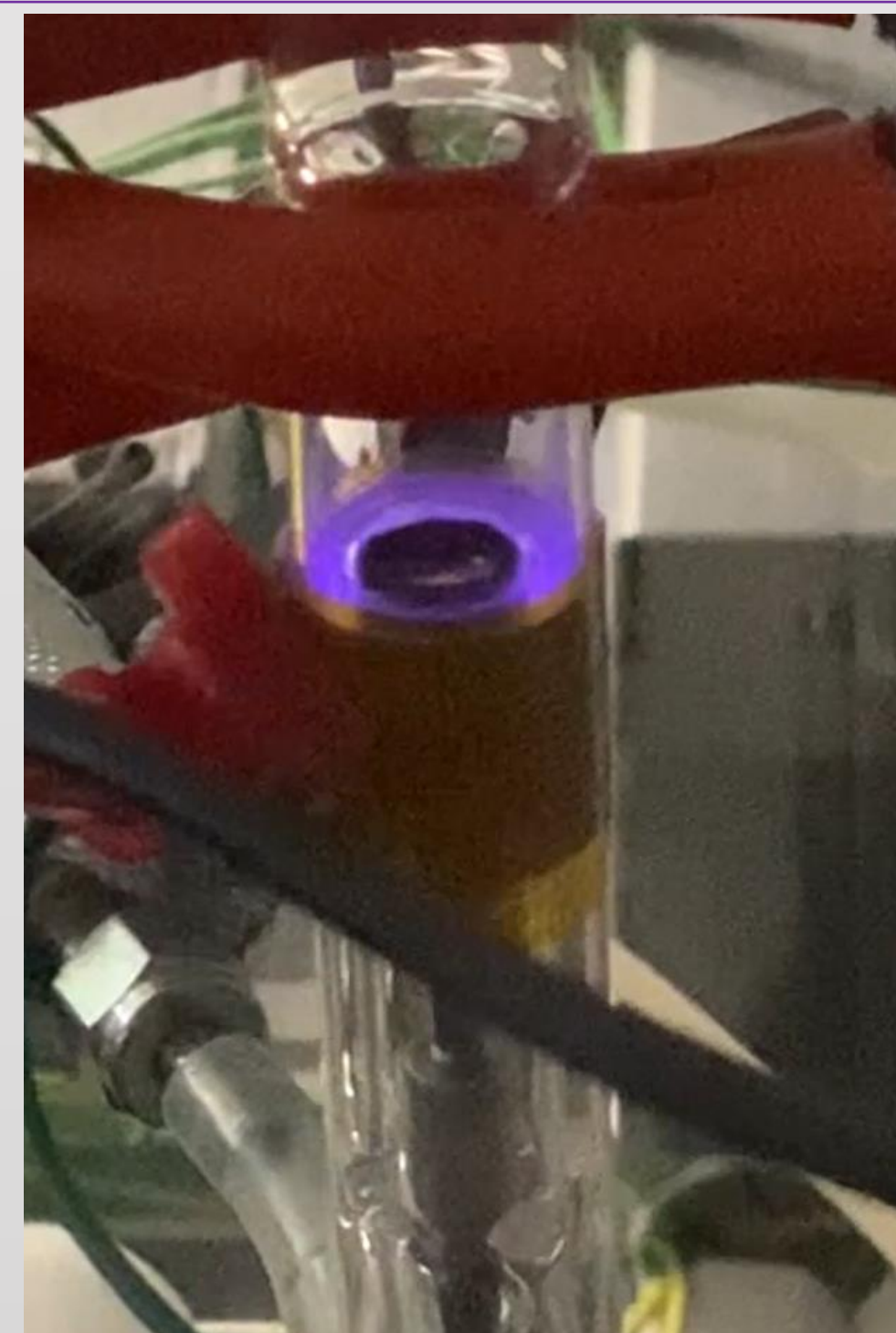
Figure 4. DBD reactor during experiment, catalyst loading inside a DBD reactor and top view of in-plasma catalyst system.
